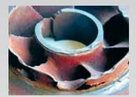
There is a picture of the cast fan of a pump exposed to cavitation on top. On the pump inlet port, abrasion on the cast fan (impeller) is clearly noticed.
